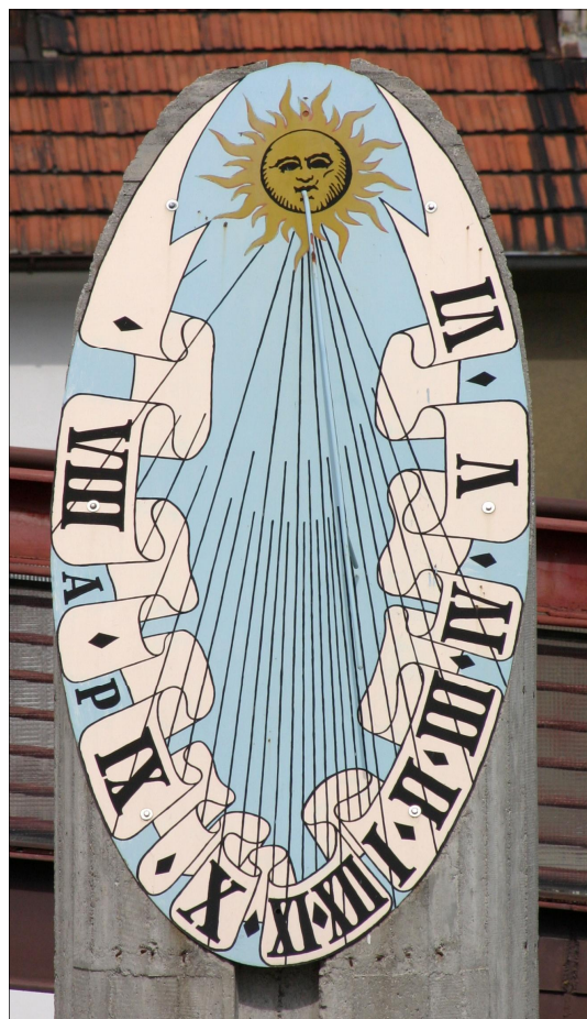
Fig. 7. Reclining dial on a concrete pillar at the roadside in Strakonice, Czech Republic.
