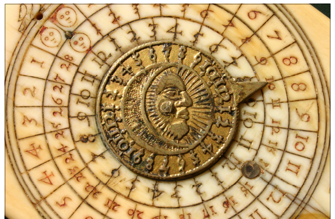
Fig. 12. Nuremberg ivory diptych dial by Hans Troschel showing the moon in the centre and three small moons punched into the ivory plate.
